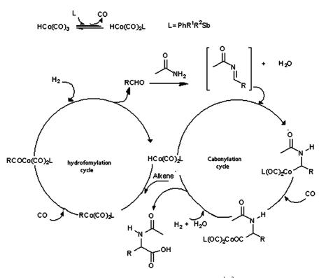
Scheme 2. Mechanism of amidocarbonylation reaction PhR<sup>1</sup>R<sup>2</sup>Sb/Co system.
